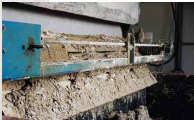
At High Concrete's plant, cement is removed by a vacuum-filtration process. The cement particles accumulate on the exterior of a rotating drum pre-coated with a layer of diatomaceous earth. The blade slices the cement off the drum, and it accumulates in a nearby hopper.
